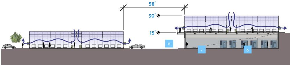
Figure A.16 Site section showing the relationship between modules. Note the lower floor may be omitted on flatter terrain
