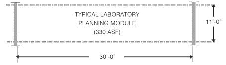
A planning module approximately 11'-0" wide by 30'-0" deep is recommended for the laboratory spaces. This module will provide adequate bench space plus space for floor standing equipment and fume hoods, and can be divided for smaller support spaces such as equipment and instrument rooms. The recommended module size will be tested against the column spacing and exterior wall locations of the proposed relocation site during the design phases, and may be adjusted accordingly.
