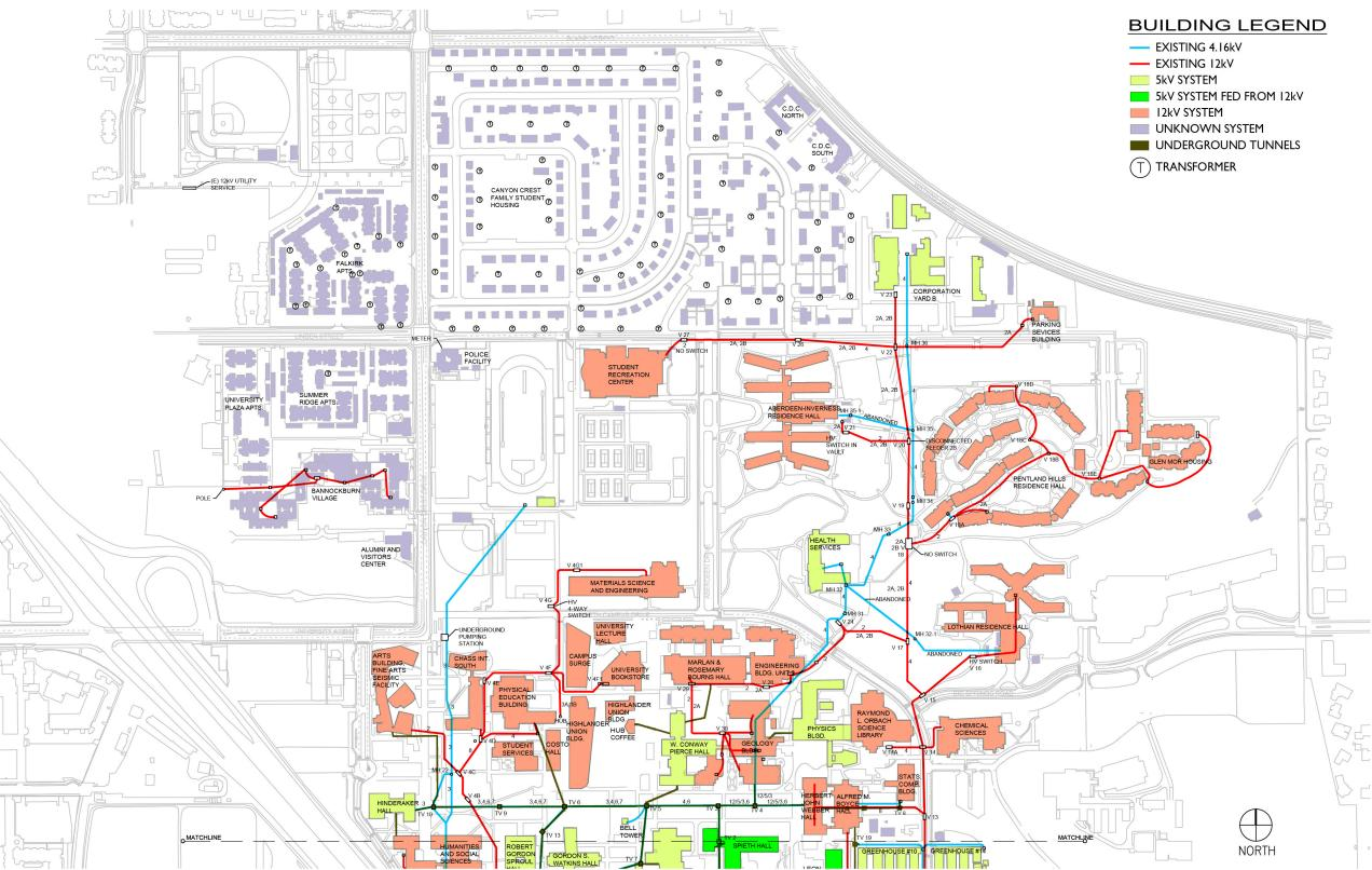
Figure 2.1—Existing 4.16kV and 12kV Electrical Site Plan by System–North
