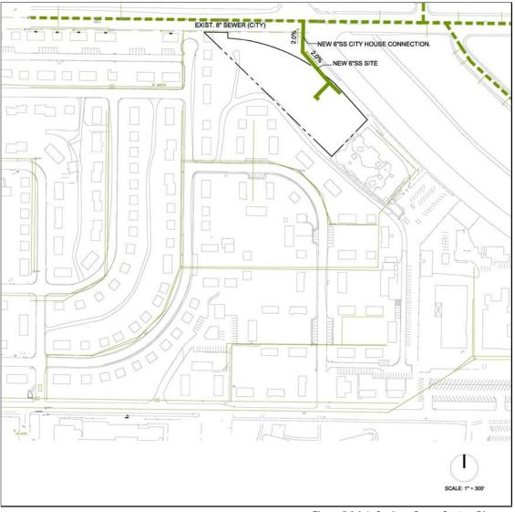
Figure 5.2.2-1: Sanitary Sewer System Diagram
